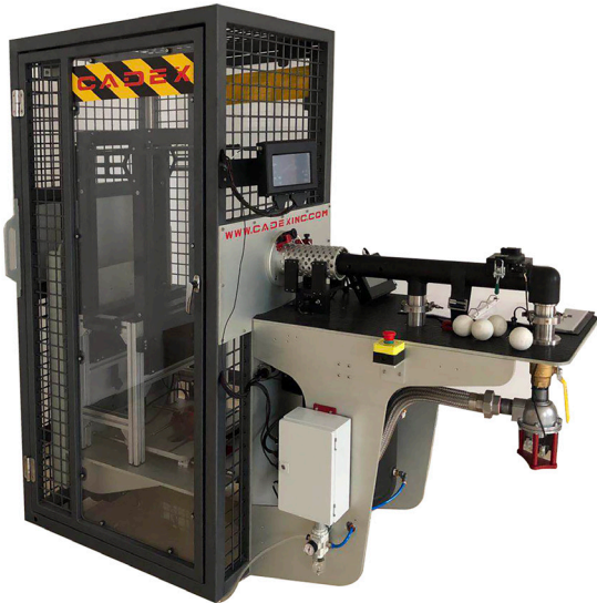
In-house COR test machine
